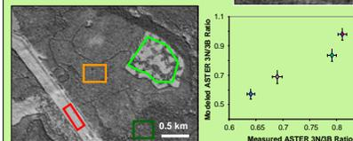
Shaded relief image produced from the LiDAR data shown above. In color - ROI's for which modeled and measured ASTER 3N/3B ratios are compared in the graph to the right
