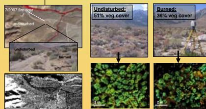
Vegetation cover is quantitatively constrained from ground-based LiDAR (5mm resolution ~100 m<sup>2</sup> maps acquired in Sep 2009 and utilized to calibrate 3B/3N ASTER ratios
