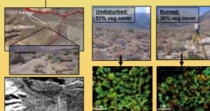
Vegetation cover is quantitatively constrained from ground-based LiDAR (5mm resolution ~100 m maps acquired in Sep 2008 and utilized to calibrate 3B/3N ASTER ratios
