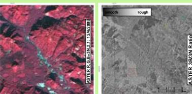
ASTER false color image for part of the Gifford Pinchot study area (left) and a 3B/3N ratio image for the same area (right). Pixels with slopes >10° were excluded from the stand-age vs. ASTER 3B/3N calibration curve shown above.
