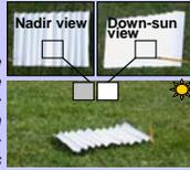
Rough surfaces appear lighter from the 'down-sun' view as shadows become progressively obscured by sunlit elements → The ratio between images acquired at such viewing geometries responds primarily to sub-pixel surface roughness
