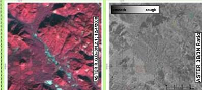
ASTER false color image for part of the Gifford Pinchot study area (left) and a 3B/3N ratio image for the same area (right). Pixels with slopes >10° were excluded from the stand-age vs. ASTER 3B/3N calibration curve shown above.
